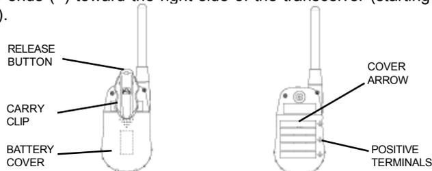
1. Using thumb, press down on battery cover at arrow and slide cover down to open.
