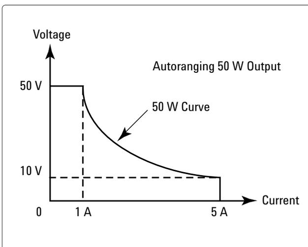
due to its extended voltage and current range, can produce voltage and current combinations in the range of a 250 W non-autoranging power supply.
