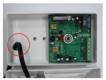
3. Connect the PIR detector power, N.O and N.C wires. Also separately connect to the camera coaxial power and BNC video connectors (observe polarity for power – connecting reverse polarity will damage the camera and void the warranty).
