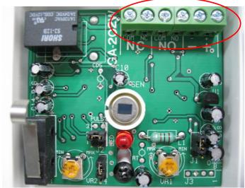
4. If not using the bracket provided (not recommended), attach the PIR detector back cover to the mounting surface with the screws provided (Do not over tighten the screws). If corner mounting the unit, drill a hole ~3/16" diameter in each edge, just below the motion detector PCB. **NOTE:** If the bracket is **NOT** used, there is no way to change the camera direction/aim the camera.
