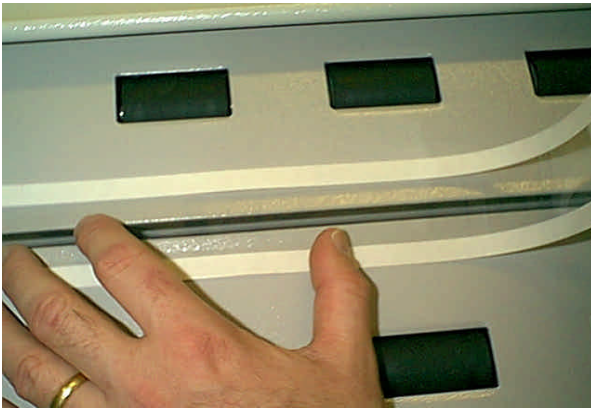
The application of Aperture Tape to the Series 4 Colortrac scanner
