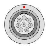
b) Power connector SATELLINE-EASy Pro 35W Connector: 4 pin ODU MINI-SNAP Style G4 size 1
