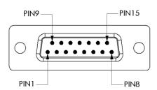
D15 female connector in radio modem.
