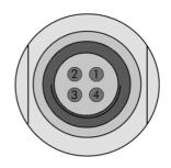
NOTE! SATELLINE-3ASd Epic Pro does not have a separate power connector. Power is fed via data connector.
