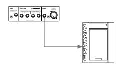
2. Connect the XLR output to the input of your PA system. The PA will see a blended signal of both Microphone and pickup. This is a great way to control exactly what the soundman has to work with and what the audience will hear.
