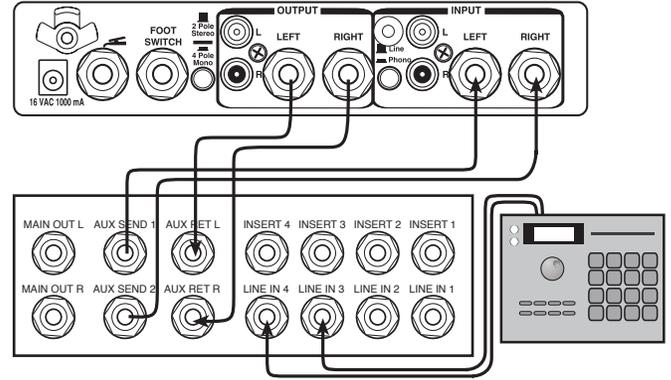
This setup requires a mixer with auxiliary (aux) sends and return capabilities. All sources are connected directly to the mixer channel inputs. Filter Queen is fed its signals from the mixer's aux sends. This setup allows any or all of your sound sources to be processed through Filter Queen at any time. The mix control on Filter Queen should be set to 100% wet so that the dry source signal is only heard through the mixer.
