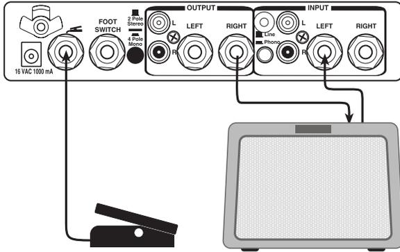
The Filter Queen can be inserted into a guitar amp or bass amp's effects loop. Use the 4 pole mono mode in this setup and experiment with Filter Queen's Effects Mix control to get the best balance between the wet, (effected) and dry signals.
