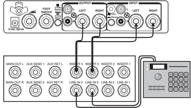
The Filter Queen can be inserted into a console's channel or bus insert just like any other outboard EQ or compressor. This setup makes for easy repatching and allows you to quickly audition the effect that Filter Queen will have on any number of sources.
