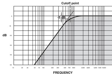
**The High Pass Filter** will roll off the bass of your signal making things sound thinner as you turn the frequency control to the right.
