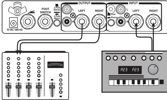
This is the most basic way to integrate the Filter Queen into any setup. In the studio this setup is a great way to warm up digital keyboards or give drum machines new life. This setup also has special advantages for live DJ's in that a turntable can be directly connected to the Filter Queen's built in phono pre-amp. With this setup the effected signal can be cued on the mixer while other sources are playing.
