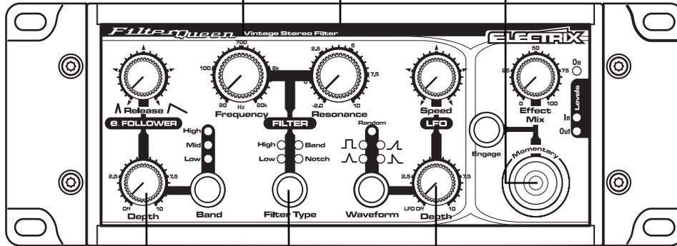
The **'Low Pass'** filter type is the standard synthesizer setting. This setting rolls off the high frequencies when the frequency control is turned to the left.
