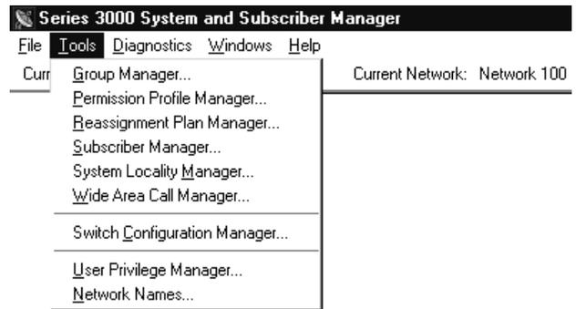
The preceding tools menu is used to select the screens for the program functions that are common to all Switches on the network. Parameters unique to individual Switches are programmed by the Switch Configuration Manager described in Section 6. The Tools screens and the section of this manual in which they are described are as follows:
