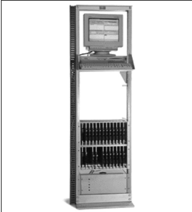
Figure 2-2 Two-Shelf Switch With CP/SSM
