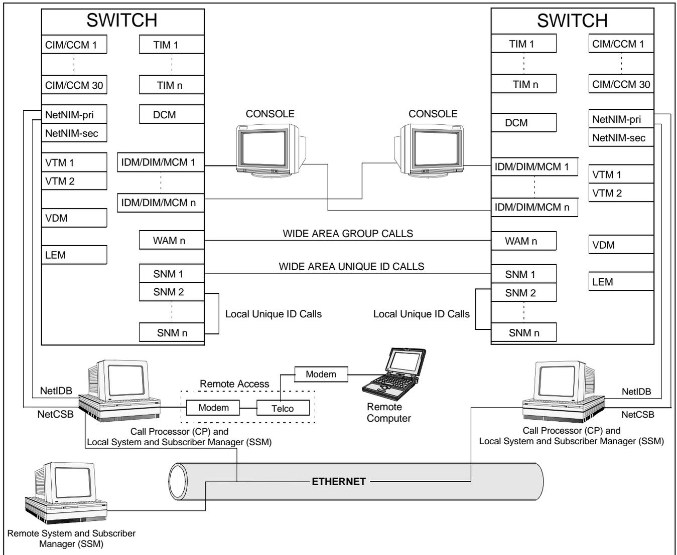
Figure 3-5 Switch Components Block Diagram
