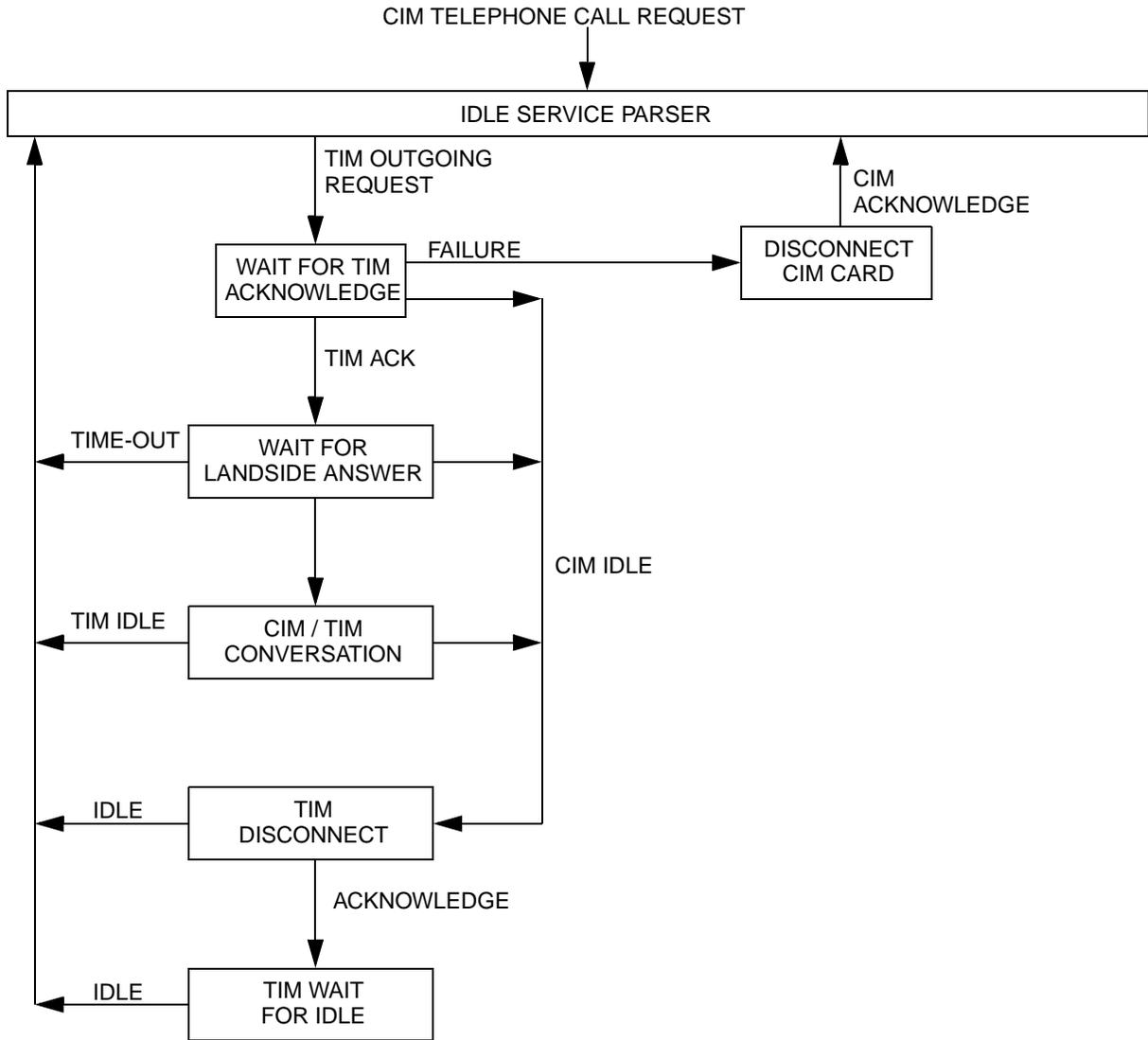
Figure B-5 Telephone Calling CIM Telephone Call Request Flowchart
