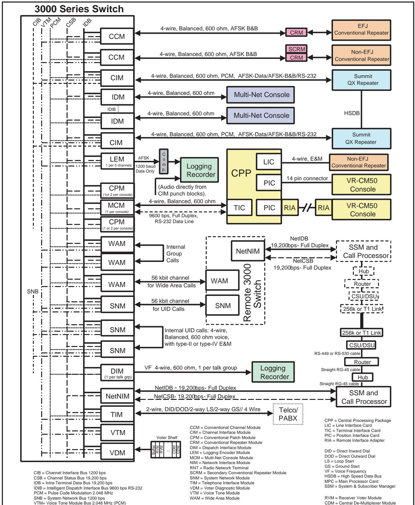
Figure 3-6 Switch Audio and Data Links
