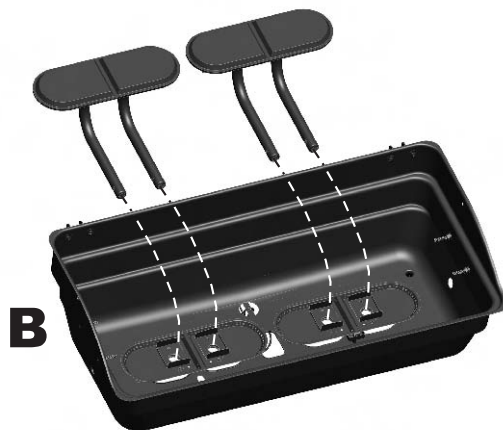
Correct burner-to-valve engagement
