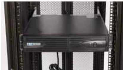
2U rackmount installation
