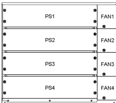
**(3) Number of installed power supply units and installation location**
