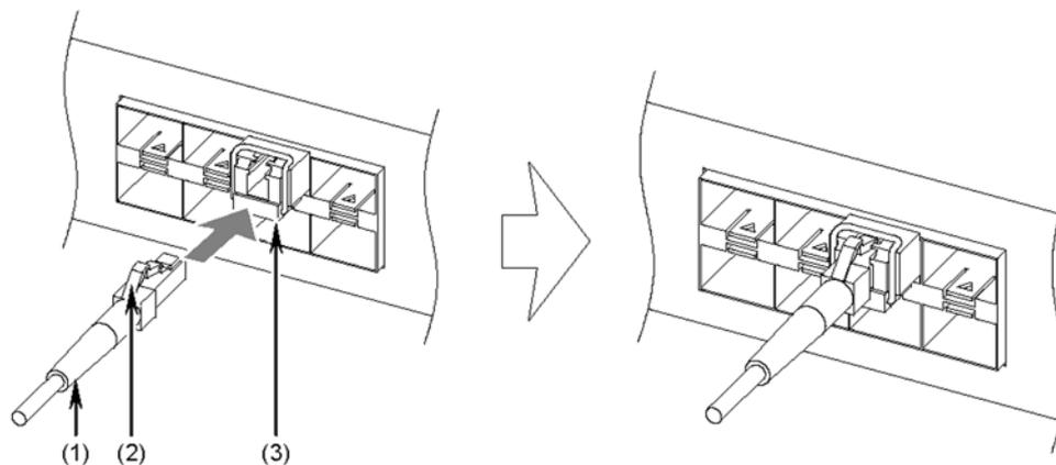
(1) Fiber optic cable (LC simplex connector)
