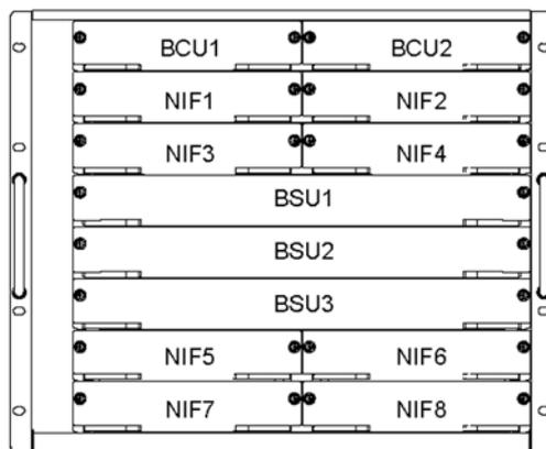
**Figure 1-5** Rear of the Switch (with an AC power supply unit installed)
