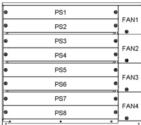
**Figure 1-6** Rear of the Switch (with a DC power supply unit installed)
