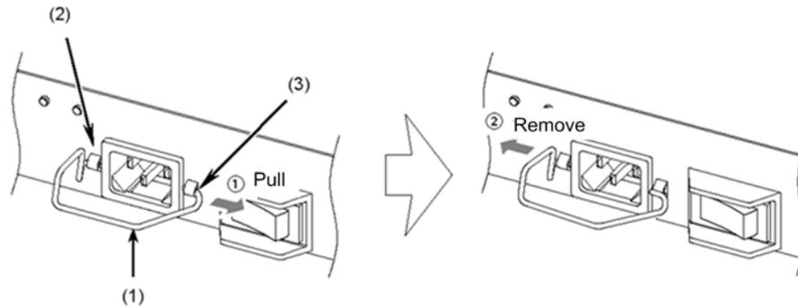
(1) Bracket preventing disconnection of the power cable
