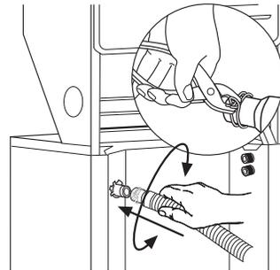
5. Place clamp over the area marked "CLAMP." Release clamp.
