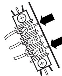
6. Tighten strain relief screws.
