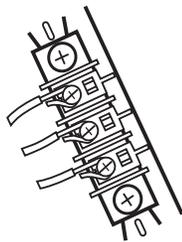
1. Remove center terminal block screw.
