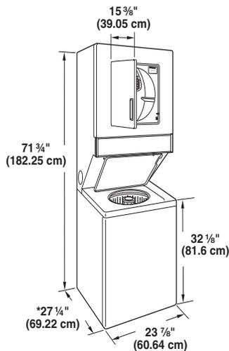
\*Most installations require a minimum 5 1/2" (14 cm) clearance behind the dryer for the exhaust vent with elbow. See "Venting Requirements."
