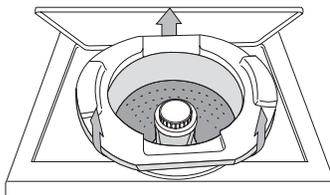
**NOTE:** Keep the foam ring and use it when transporting your washer/dryer. This packing material is used to keep the washer tub stable during transport.
