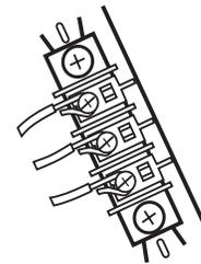
1. Loosen or remove center terminal block screw.
