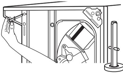
2. Check adjustability of rear legs by pushing in one leg. The other leg should come out. Check both legs. If they do not move freely, repeat Step 1.
