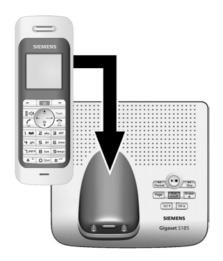
To start the automatic registration of your handset, please place the handset in the base with the display facing outwards. The handset registers automatically. Please do NOT remove your handset from the base station during the registration procedure.
