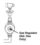
Connection to the gas supply should be made using the Aquaknect AS/NZS 1869 class B hose assembly with an internal diameter of not less than 10mm and regulator (regulator for use with natural gas)
