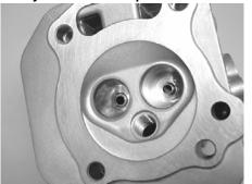
bowls. Pay special attention to the intake runner where it enters the bowl as it is offset to promote swirl and needs to retain the offset in order to maintain the swirl characteristics. Next mount the intake manifold to the head and blend the junction. The outlet of the manifold has been purposely left a little undersize so that it can be increased to match the head.
