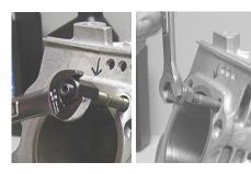
• Stud Installation: Apply a small amount of (blue) Loctite to the threads of the dimpled end of the stud and install using a stud driver as shown. (see "Special Tools") Note-there are two different ends to the studs; dimpled and rounded—install the dimpled end in the block. Run the stud down until it lightly bottoms and tighten it ¼ turn more. (An
