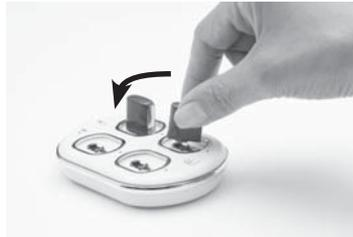
1. Remove the rechargeable battery module from the processing unit.
