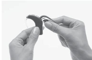
1. Carefully lift the accessory socket cover of your processor with a screw driver.
