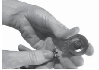
1. Hold the coil and coil cable with the underside of the coil facing up. Pushing your fingernail between the coil and coil cable on the underside of the coil may help detach the coil from the coil cable.
