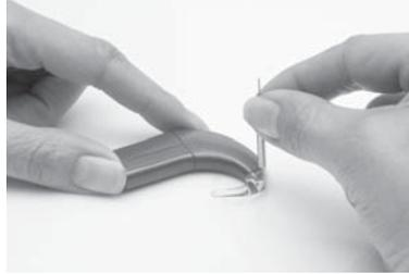
1. Attach the tamper resistant earhook to the processing unit. Ensure that the hole on the earhook is aligned with the hole on the earhook end (tip) of the processing unit.
