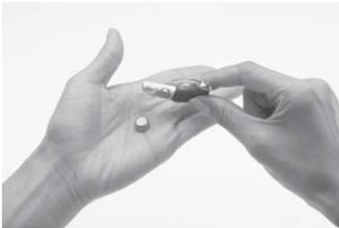
3. Remove the disposable batteries (zinc air batteries) from the battery holder.
