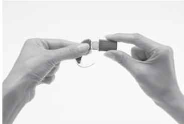
4. Replace the battery cover by sliding it up from the bottom of the battery holder towards the processing unit. Do not force the cover upwards as it should fit easily.
