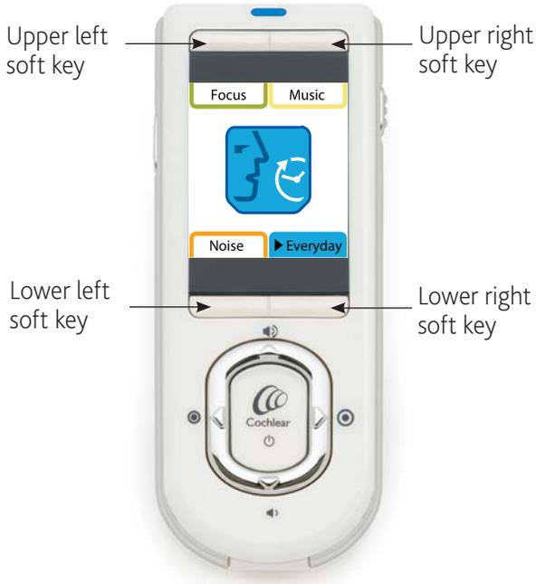
Figure 17: Soft keys for selecting a program from Home screen
