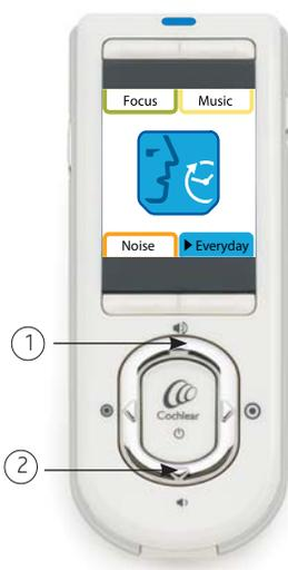
Figure 20: Directional keys for increasing volume (1) and decreasing volume (2)
