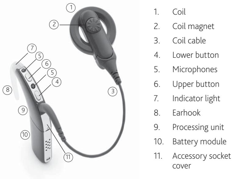
Figure 1: CP810 Sound Processor parts
