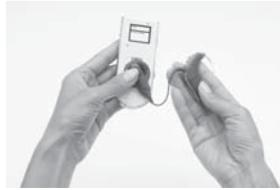
Figure 14: Placing the coil on the back of the remote assistant
