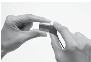
3. Insert the battery module into the LiteWear Case by gently pushing on the lower end of the cable shoe. The Battery Module can be inserted both ways.
