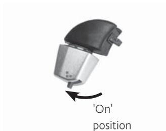
Figure 25: Phonak receiver connected to the Euro Accessory Adaptor
