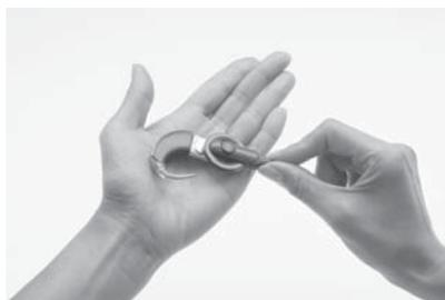
1. Place the coil magnet over the batteries so that the coil magnet touches both batteries. The coil magnet will lift both batteries out of the battery holder.
