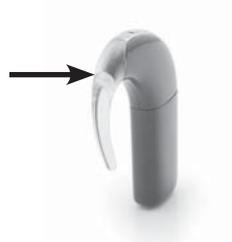
1. Remove the earhook from the processing unit by pushing the lower end of the earhook towards the processing unit.
