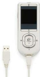
2. Plug the other end of the CR100 Series USB Cable into the CR100 Series Global Power Adaptor.
