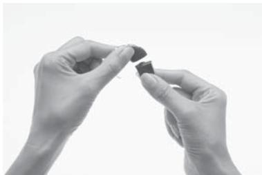
1. If the battery module is attached to the processing unit, detach it from the processing unit.
