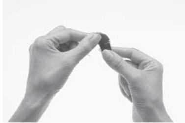
1. Hold the battery module and the processing unit so they touch. The battery module should face to the left and the processing unit to the right of the final position.
