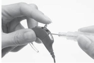
1. Attach the LiteWear Cable to the processing unit.
