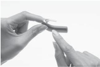
3. Make sure the battery module is correctly aligned. Check for broken or bent contacts between the battery module and the processing unit, which can cause misalignment. If any contacts are broken, return the processor to your clinician.
