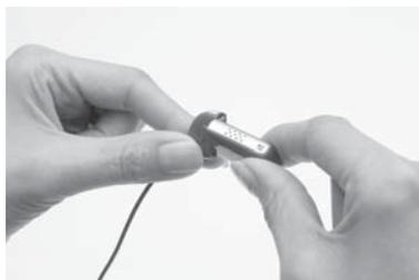
4. Hold the battery module and the lower shoe of the LiteWear cable (cable end that connects to the battery module) so they touch. The lower shoe should face to the right and the battery module to the left of the final position.
