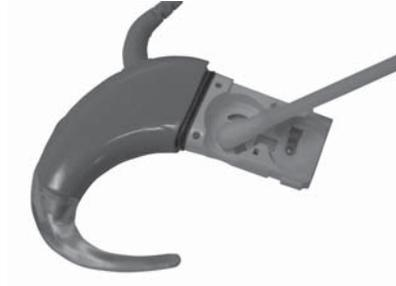
1. Remove the batteries from the battery holder.
