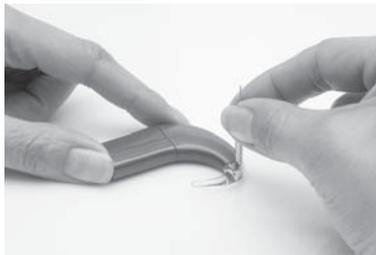
4. Push the earhook fitting pin in with the earhook fitting tool until the pin is fully inserted. Ensure that the pin does not protrude from either side of the earhook.
