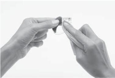
4. Wipe the battery holder and battery cover (inside and outside) with a soft dry cloth to remove any water, moisture or sweat.
