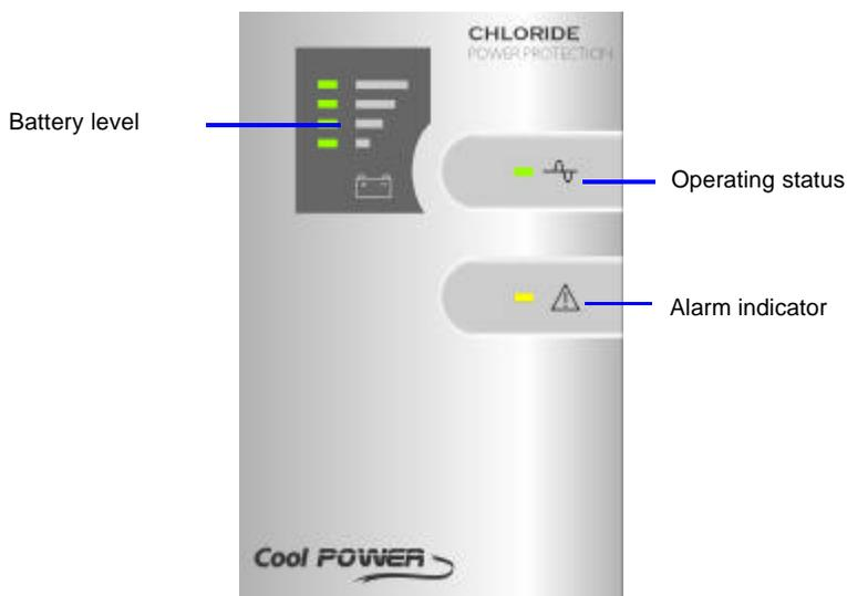
1. Battery level : Indicates the charge level of the battery. For more information see Part 5.2.
