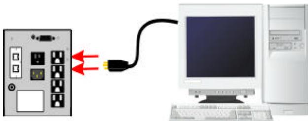
2. Connect the selected load (i.e. printer, scanner) to the surge protected outlet. Appropriate loads are those elements that demand surge protection, but that do not require extended runtime during power outages.
