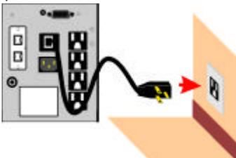
6. Once connected to the mains, check to make sure that the LED on the front panel is green within a few seconds. Immediately after connecting the UPS to the AC network the equipment runs a self-test. If the test is successful and the electricity supply is within the specified limits, the equipment will start up and will supply energy to the output connectors.
