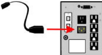
5. Plug the power cord into the mains. The computer's power cord may be used.
