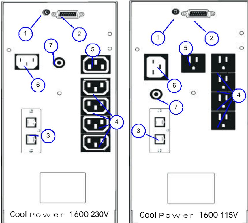
1. Battery test : This button enables you to run a battery test, switch off the UPS and restart it without mains electricity. For more information see Part 5.3.
