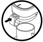
3. **Slide Pod Drawer into Drawer Guides and push in to lock into place.**
