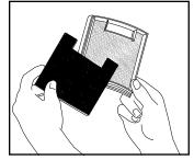
Remove foam from filter frame. Shake filter frame and foam filter to remove excess dust.
