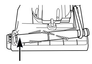
Remove the hood from the cleaner and check for a blockage in the brush roll area. Make sure the hose inlet is clear. If no blockage is found, continue to step 4.
