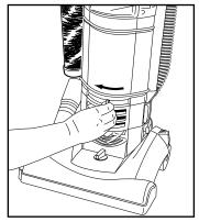
Remove dust cup by sliding dust cup lever from right to left.
