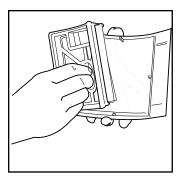
When dry, replace foam filter into filter frame.
