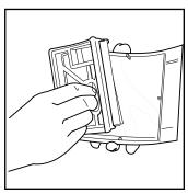
Remove filter frame from top filter cover.
