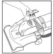
Replace filter into unit. Replace bottom filter cover by pivoting back onto cleaner from left to right.
