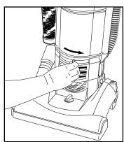
Replace dust cup lid, reposition in cleaner body and secure by moving lever from left to right.
