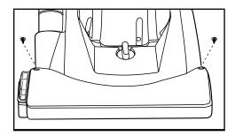
2. Remove the two screws from the top of the hood.
