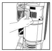
Replace filter frame into top filter cover. Replace top filter cover by pivoting back onto cleaner from left to right.
