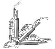
Handle Release. Step on handle release to pull handle back to a comfortable operating position. To lower handle completely to the floor, depress handle release a second time.
