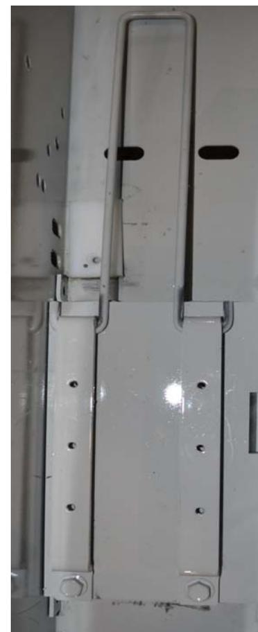
Fig 2. Safety brake deployed.
