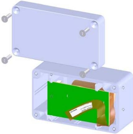
1. Locate the RF transceiver on the bottom slat (shown to left)
