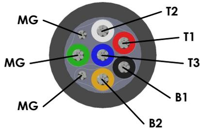
NOTE: TO CHANGE DIRECTION OF MOTOR ROTATION – SWITCH T1 AND T2
