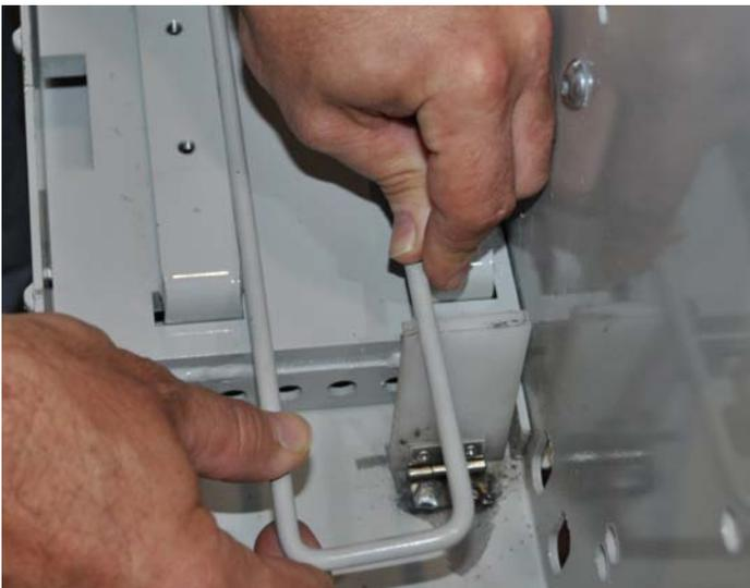
Rotate yoke rest to a horizontal position and snap yoke into pocket.
