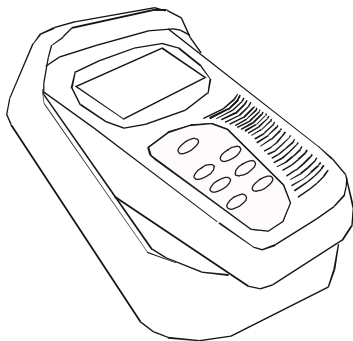
Figure 3: Inserting meter into the rubber boot
