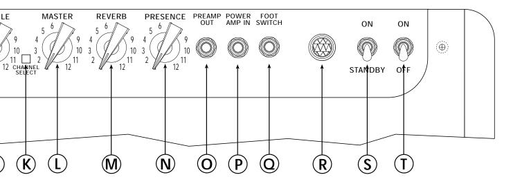
**K. CHANNEL SELECT** - When this button is pressed, the amp switches from the NORMAL channel to the DRIVE channel.
