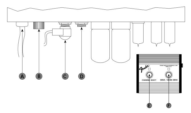
**A. LINE CORD** - the Hot Rod Deluxe is equipped with a grounding type supply cord to reduce the possibility of shock hazard. Be sure to connect it to a grounded AC receptacle. **DO NOT ALTER THE AC PLUG**.
