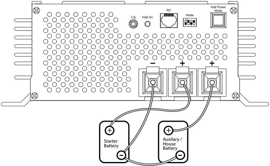
Fig. 7.1 Connecting 2 separate battery systems to 2 separate banks
