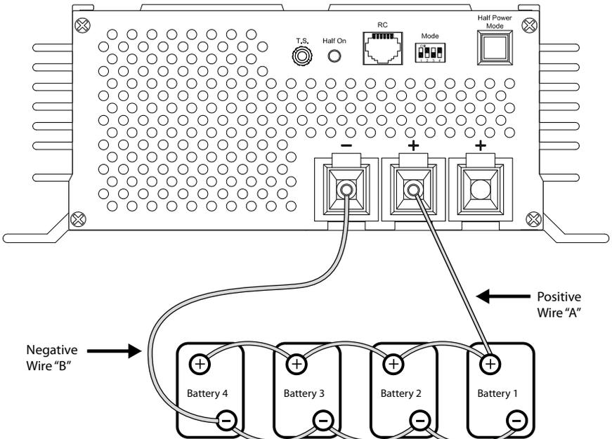
Fig. 7.2 Connecting bank of paralleled batteries to single bank
