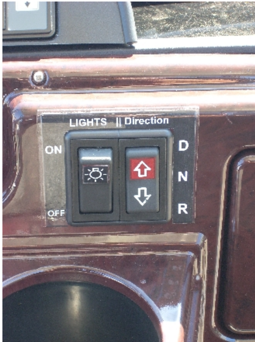
(Direction Switch shown in "Neutral" position)
