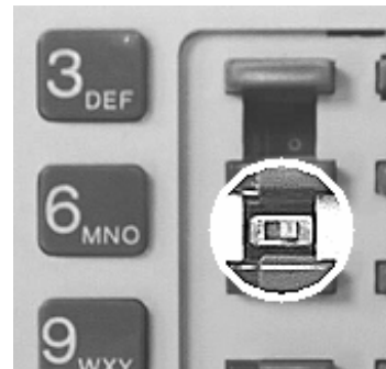
Dip to right: the 1 st station. Dip to left: the 2 nd station.
