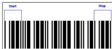
A code of code type *Codabar* can have one of the four characters (A, B, C or D) as the start/stop character. If only identical start and stop characters are permitted, the reading reliability is increased, and misinterpretations are avoided.
