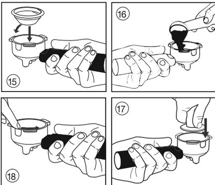
**IMPORTANT:** Be sure not to overfill the filter basket with coffee as this can cause the portafilter holder to leak or overflow
