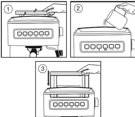
4. To fill the espresso machine with water, simply lift the lid of the water reservoir at the top of the espresso machine, (1) and fill with fresh cold water or filtered water (2) or remove the reservoir and place the water reservoir down firmly until the reservoir cover is flush with the top of the espresso machine (3).
