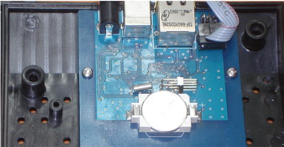
**Fig.4. The coin battery cell is located at the centre of the circuit board of the BS1000.**
