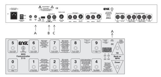
1. MIDI foot board (for example, the ENGL Z-12 or ENGL Z-15 pictured above): Connect the foot board to the amp using a standard 5-pin DIN cable. All 5 terminals of both connectors must be wired in a 1:1 configuration: MIDI data transmission requires two wires, and the ENGL MIDI foot board uses two more wires for purposes of power supply. This combination affords access to all of the amp's 128 MIDI presets.
