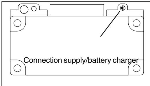
When using the power supply/charger unit you are able to simultaneously charge NiCd cells in the USN 52 R and operate the instrument. The power supply/charger unit requires 4 to 7 hours in order to fully charge the NiCd cells.
