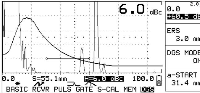
The **GAIN** function shows the incremental and reference gain, e.g:
