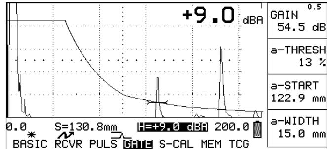
The recording threshold violations in dB can also be easily determined:
