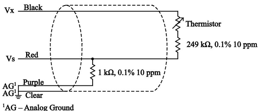
FIGURE 8-1. 107 thermistor probe schematic
