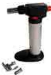
4 IN 1 BUTANE TORCH 8257-31 Use as a torch, soldering iron, hot air blower or shrink tube tool.
