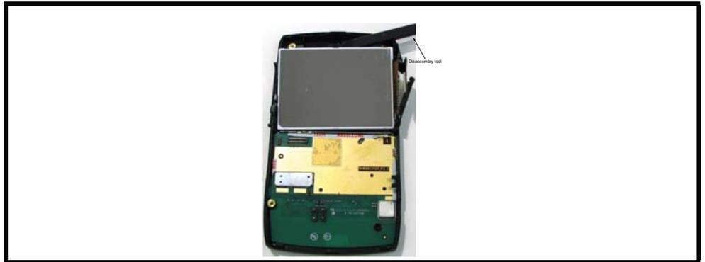
**Figure 26. Removing the Display Module**
