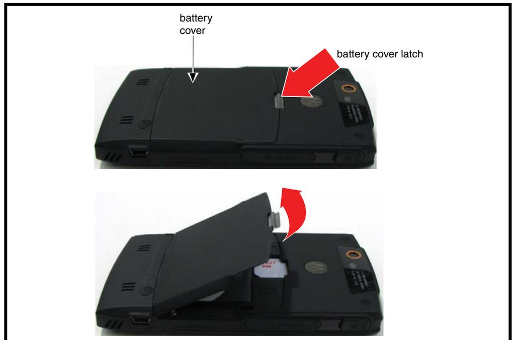
Figure 1. Removing the Battery Door
