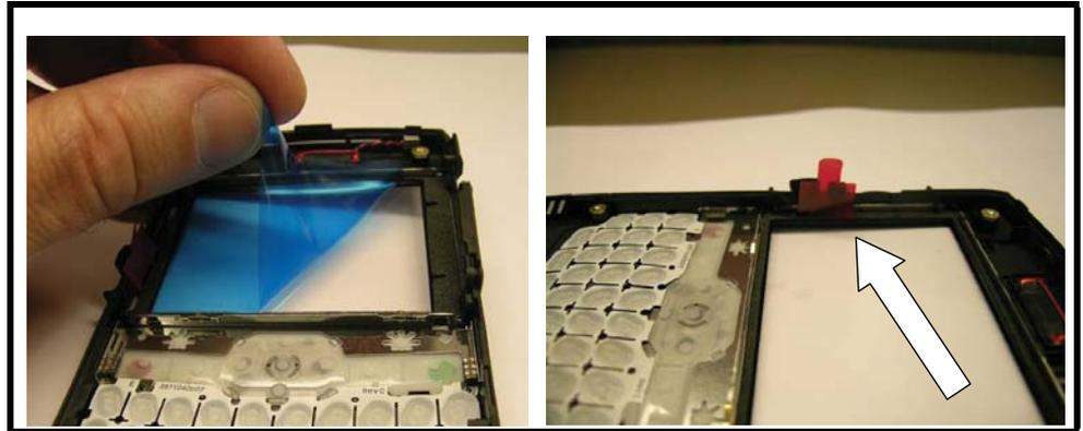
**Figure 28. Removing the Protective Liners**
