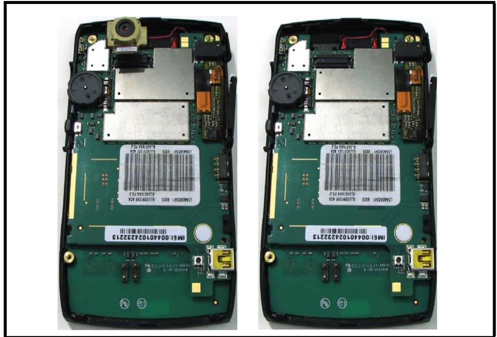
**Figure 12. Camera Assembly Removal**
