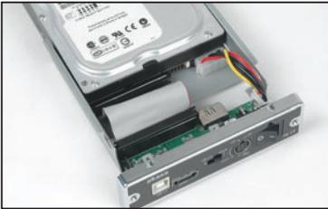
3. Place the HDD in the tray aligning the correct IDE and power connectors. Then connect the IDE and power connectors to the HDD.
