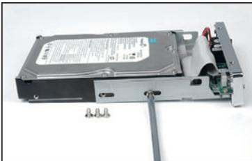
4. Position the HDD in the tray so that the mounting holes on the HDD line up with the tray mounting holes. Use the four screws supplied in the mounting kit to secure the HDD in the tray.
