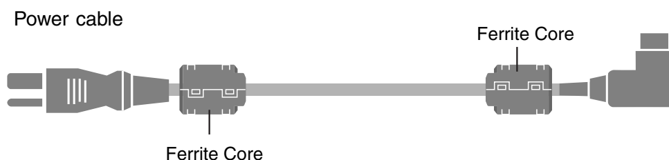
Figure 4-1. Attaching the Ferrite Cores to the Power Cable
