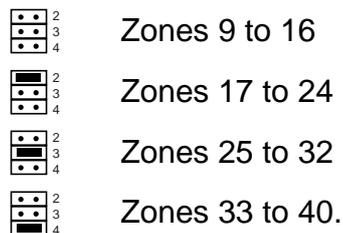
Figure 25. Link Positions to Allocate Expanders to Zones
