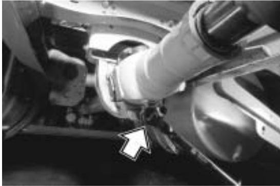
**54****Check Drive Shaft, Universal Joints, Sliding Joints and Support Bearings**
