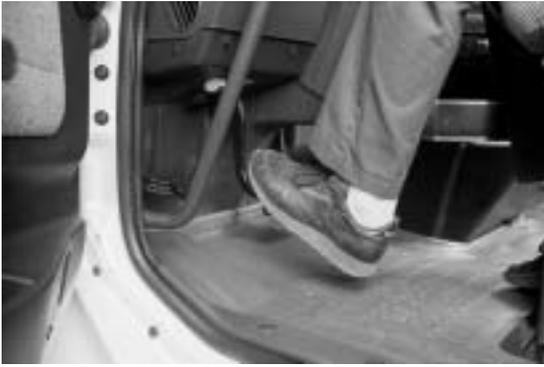
**27****Check Gear Shift and Clutch Pedal**
