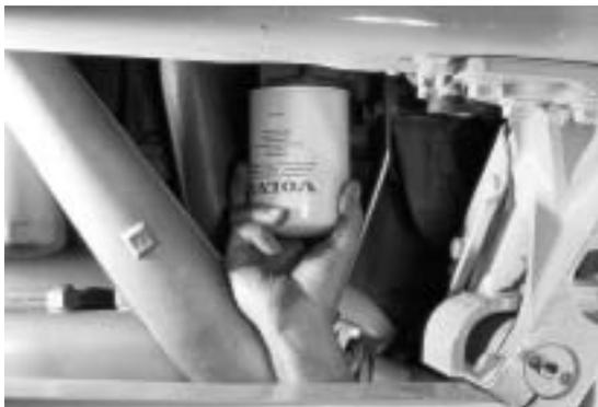
Draw coolant for testing. Adjust coolant as necessary and change the filter if needed.
