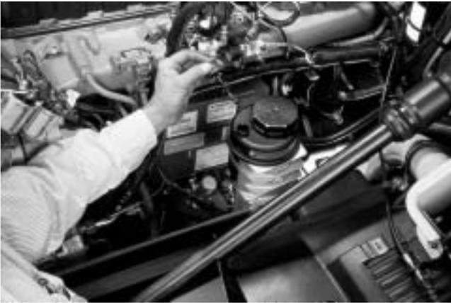
Check all fluid levels. Make sure there are no signs of leakage after changing oils or filters.
