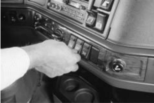
**69****Check After Test Driving****Check Pneumatic Switches**
