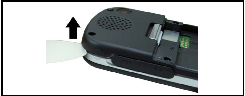
Figure 9. Prying open the back cover
