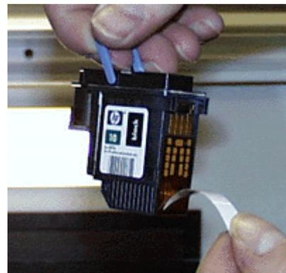
11. Insert the new print head and push down firmly on top to make sure print heads is seated properly in the carriage. Close and latch the printhead clamp. Push head release lever forward towards you.
