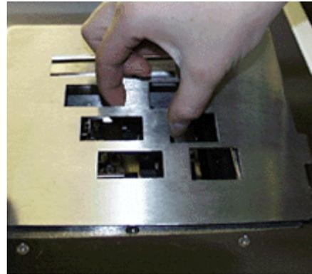
4. Squirt distilled water onto the squeegee and wipe clean with the small brush provided with your Z406 3D Printer until all debris is removed.
