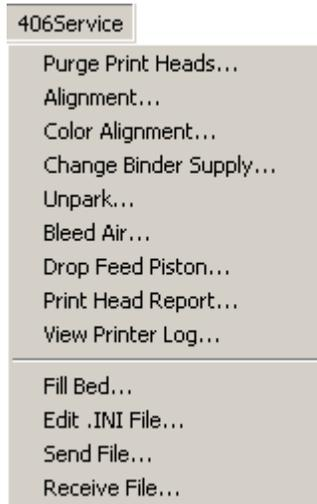
1. Make sure you have run through the standard alignment, purged the print heads, and changed the binder supply to color mode.
