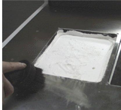
7. Spread the gantry so that it is above the feed piston. Press and hold the Feed Up Button until the surface of the powder is even with the Top Deck.
