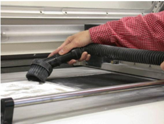
2. To prevent material contamination vacuum off any remaining powder from the feed and build plates, and the top deck.
