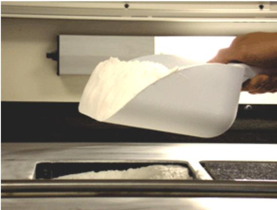
1. Remove all powder from the feed and build envelopes. Place powder in a sealed container to prevent absorption of moisture into the powder.
