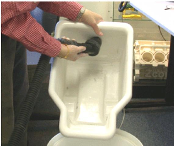
4. To prevent any material contamination, vacuum any remaining powder in the Overflow Bin.
