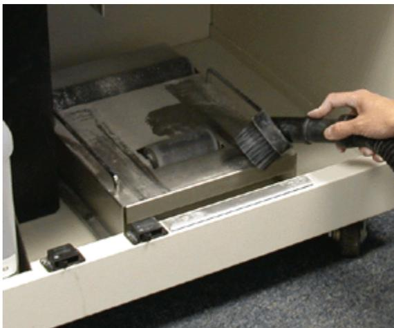
5. Before replacing the Overflow Bin, vacuum the Overflow Bin track. Then replace the Overflow Bin.
