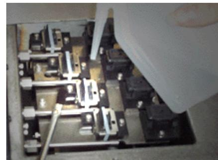
5. Squirt the distilled water onto the parking caps and wipe clean with the small brush until all debris is removed.
