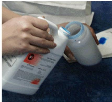
**WARNING: Do not recycle waste solution. The waste is contaminated with powder and use of this waste in the Z406 3D Printer will clog the fluid system. Use only binder supplied by Z Corporation. Use of any other material may impact the performance and safety of your Z406 System and will void warranty.**
