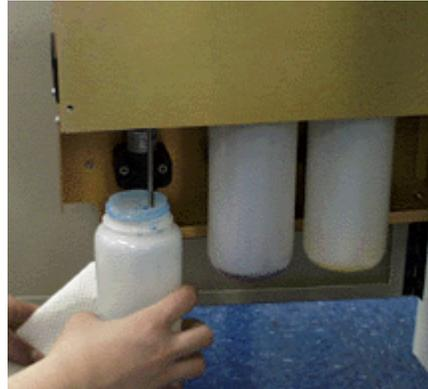
5. Fill the bottle up with binder. Replace binder bottle in the proper order – cyan, magenta, yellow (from front to back).
