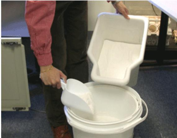
3. Remove the powder from the Overflow Bin and empty into a sealed container.
