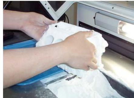
**WARNING:** When performing any vacuuming operation, use the vacuum provided as part of the Z406 System. Vacuuming powder can generate static electricity, and use of a non-grounded vacuum will create static charges, which may affect the operation of the Z406 System and harm the operator.
