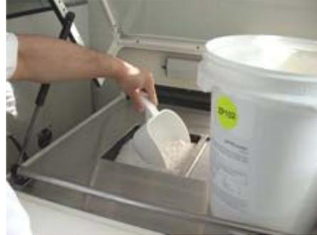
2. Carefully scoop powder from the bucket and place in the feed piston.
