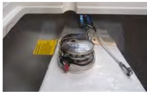
Windlass anchor roller, as seen from the anchor locker
