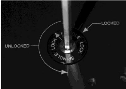
To unlock your lift turn lift handle counter-clockwise to the "UNLOCKED" position
