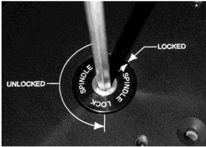
To lock your lift turn lift handle clockwise to the "LOCKED" position
