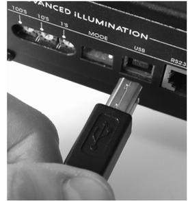
Figure 6: USB type B connector
