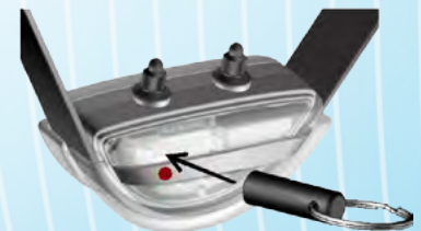
Diagram 5 Activate / deactivate the EF-6000 collar with the magnetic key
