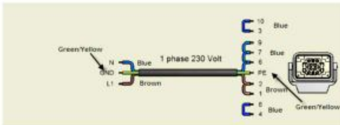
USA cable, single phase
