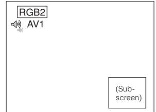
AV1: Displays the VIDEO input signal of the sub-screen.
