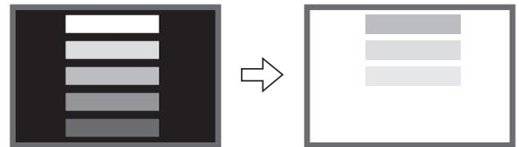
\* The image retention images in this document are exaggerated for the purpose of explanation. The actual manner in which the image retention is seen differs depending on the operation time and brightness.
