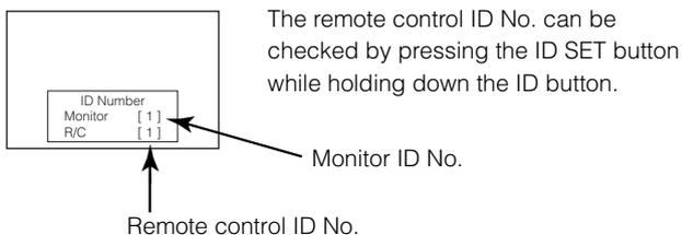
The remote control ID No. can be checked by pressing the ID SET button while holding down the ID button.
