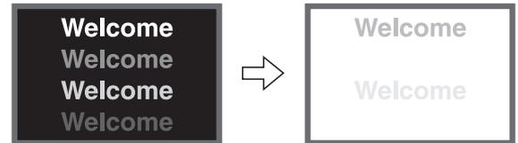
■ The degree of image retention is proportional to the brightness of the characters and figures displayed as well as the display time.
