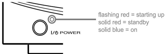
To change from the ON mode back to the standby or “sleep” mode, press the Power button on the front panel or on the remote once. The video output will go blank and the LED will be solid red.
