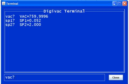
Press carriage return or enter to submit the query or change the set point. Note that while the web terminal is open, the main 200 Pirani screen will not update. If at any time the web terminal or the main 200 Pirani applet window becomes unresponsive, close the browser (not just reloading the tab or closing the tab) and reconnect.
