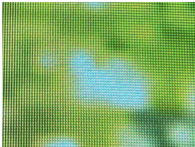
Figure 2: The “screen door” effect seen in DK1.
