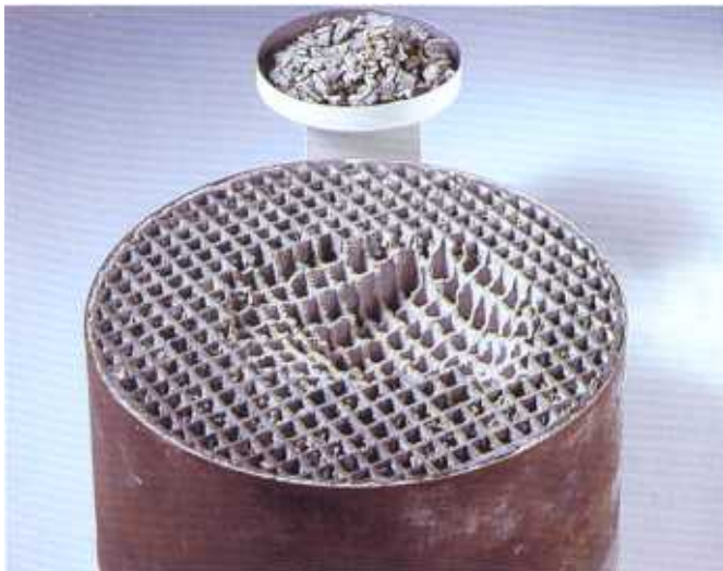
Photo #11 Substrate Crumbling (Model 6000)
