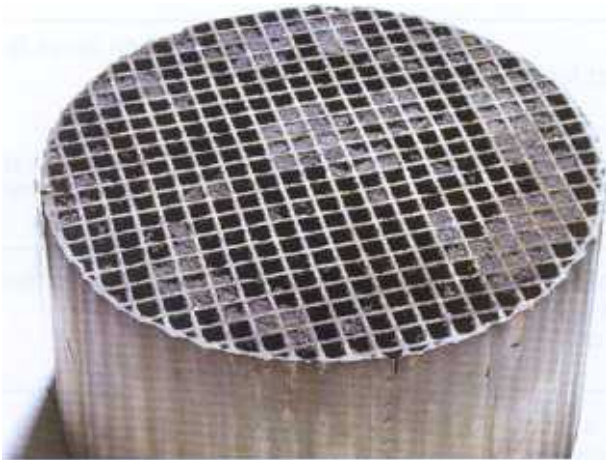
Photo #3 Creosote Plugging
