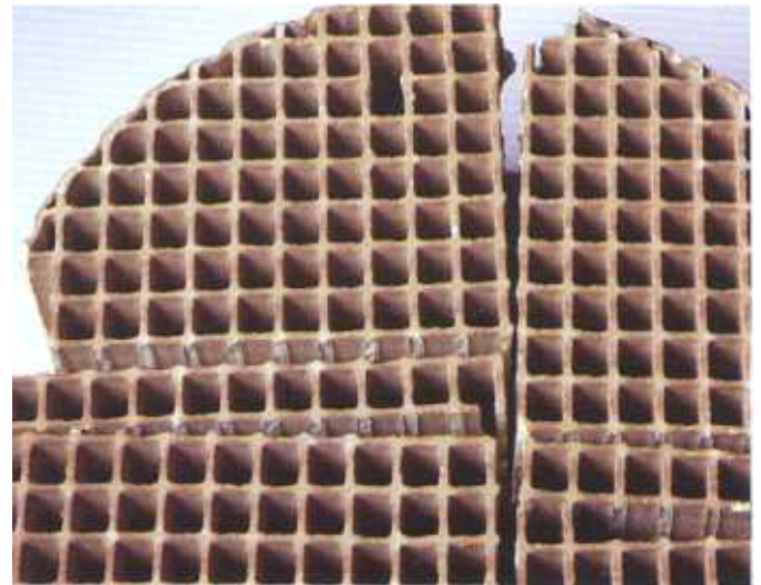
Photo #10 Mechanical Cracking
