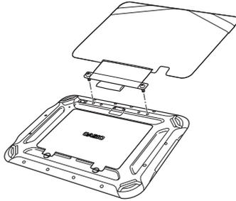
2. Close the cover so that it fits snugly against the display and fix in place by pulling the rubber bands around the back of the tablet.
